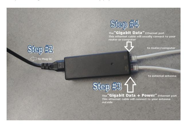
Step 3: Plug in the Ethernet cable that comes in from the outside antenna into the "Gigabit Data + Power" Ethernet port
